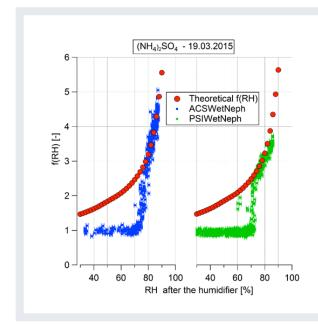
Ammonium sulfate particles light scattering enhancement (f(RH)) calculated (red markers) and measured by the ACS™ 1000 (blue dots) and the WetNeph developed by the Paul Scherrer Institute (green dots). The errors bars represent the precision of the RH measurements according to the manufacturer.
