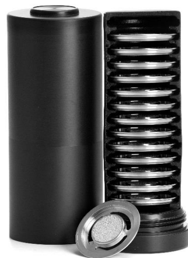
Figure 3. Set of sintered collection plates for ELPI+™.
