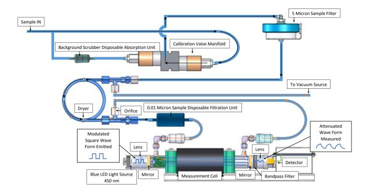
Sample air is filtered to remove particulates and dried before entering the precision stainless steel 264 mm measurement cell.
